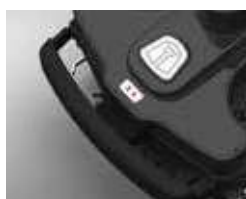
Paraurti e sensore ostacolo morbido Bumper and soft obstacle sensor
